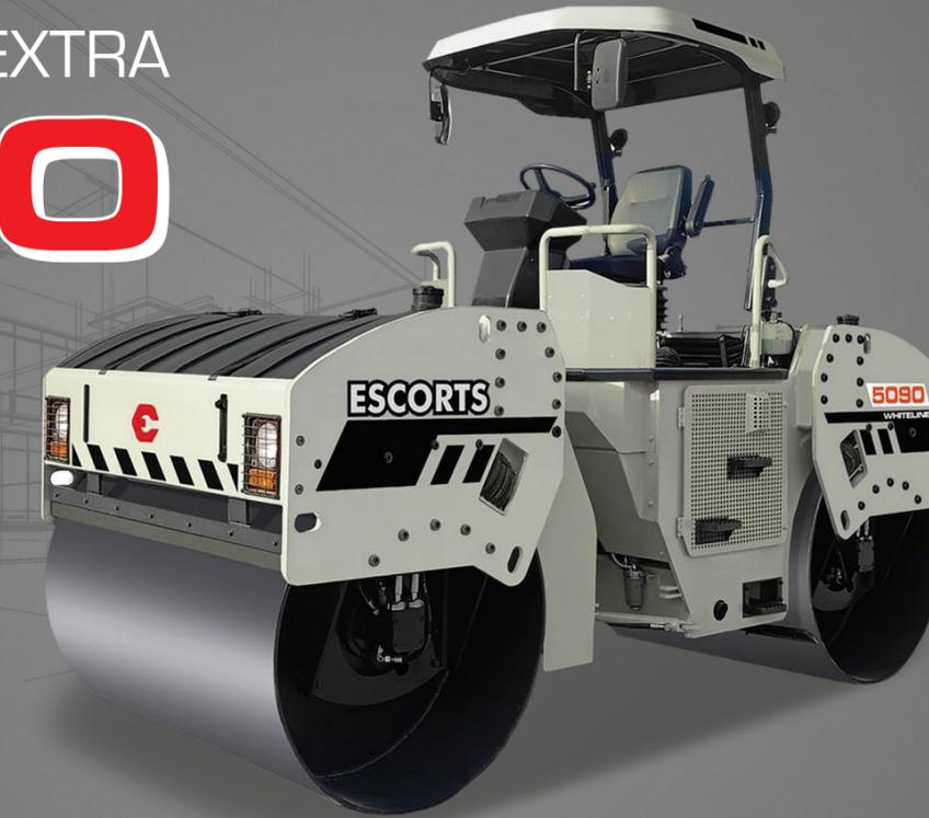
Escorts Engine: 75 HP | Static Linear Load 27.7 kg/cm | Total Applied Load 22.4 Ton
